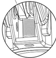
Check the screw thread. Adjust the screw clockwise, the thread becomes longer, and the load is lighter. Adjust the screw anti-clockwise, the thread becomes shorter, and the load is heavier. You may need to adjust several cycles to get to perfect position.
